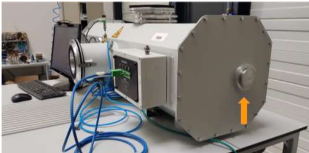
Image 4: side inlet for testing diaphragm meters
